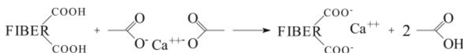
Scheme 2 Determination of the IEC by reaction of calcium exchange with carboxylic functions of treated polyester fabrics. Acetic acid formed is back titrated.
